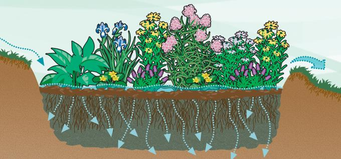
A rain garden slows the flow of rain water runoff.
